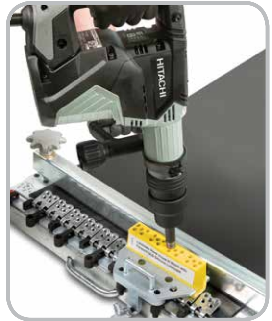
Electric Powered Rivet Driver Installation
